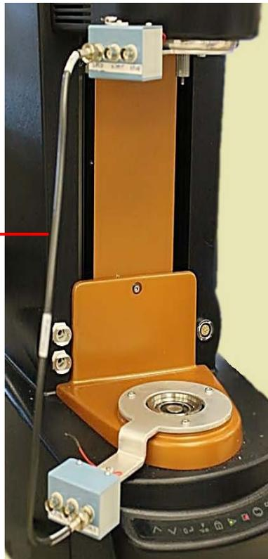
**Figure 11** Shield cable connections.
