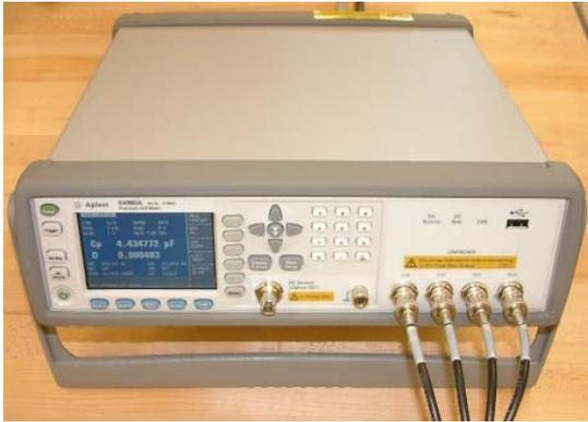
**Figure 10** The Agilent E4980A LCR Meter.
