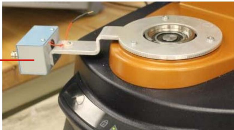
**Figure 7** Lower BNC junction box installed on the mounting base.
