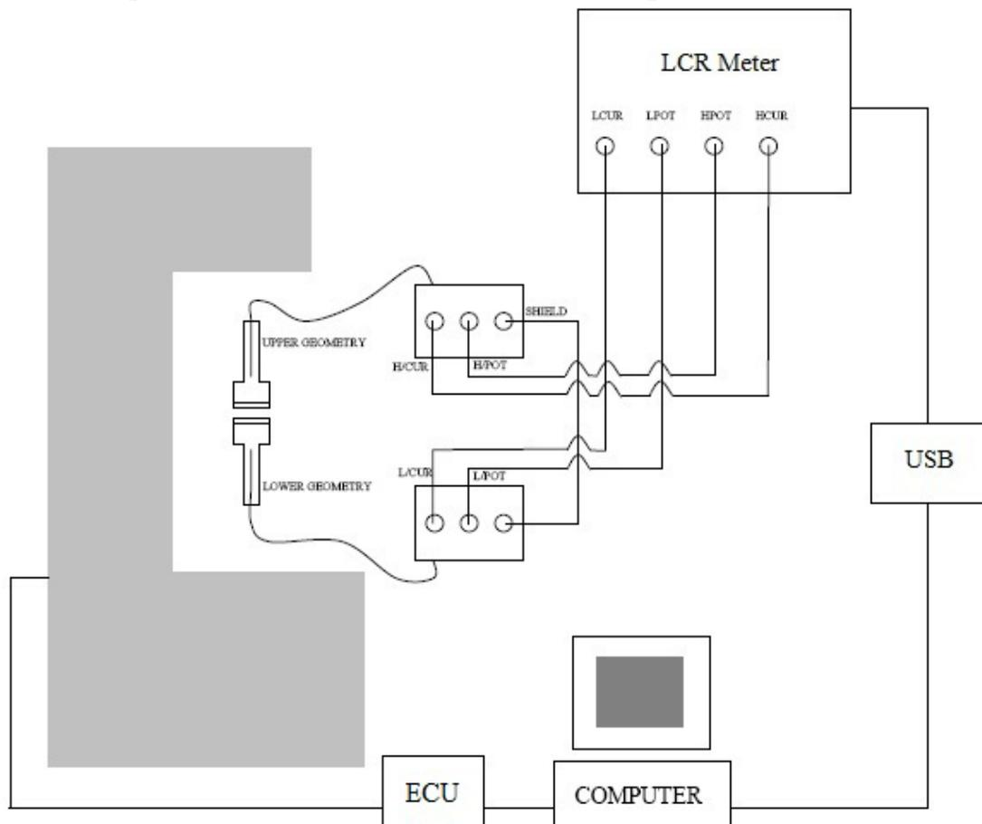
**Figure 12** Main BNC wire harness connection block diagram.
