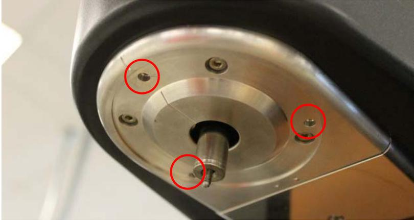
**Figure 3** Mounting ring for upper BNC junction box.
