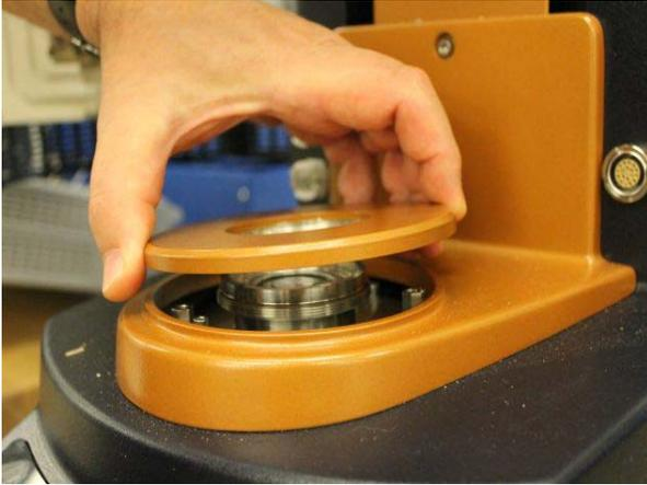
**Figure 5** Base cover unscrewed to expose the mounting surface for the lower BNC junction box support ring.
